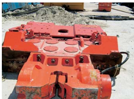
The driving gear consisted of a vibratory hammer...
