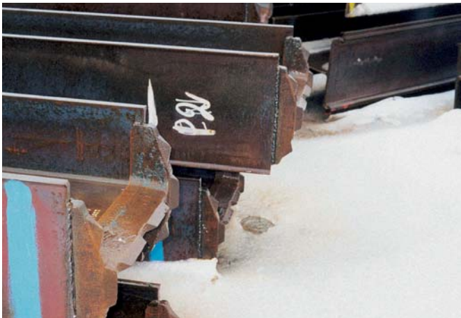
Driving shoes protect the pile toe from damage when hard soil layers are expected during driving
